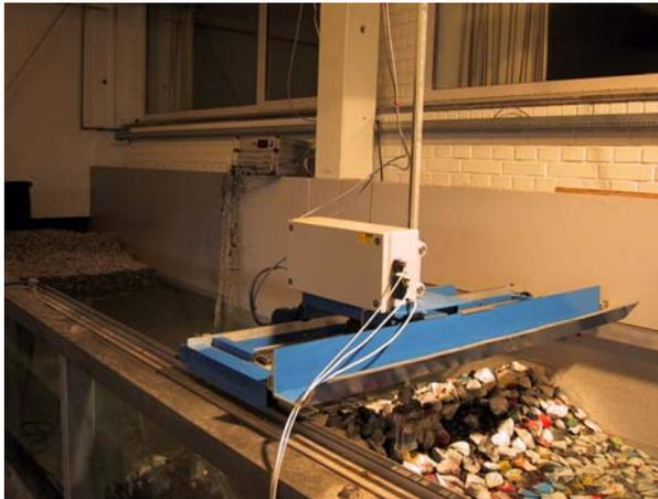
In order to avoid slipping, tooth belts are used for power transmission, hereby ensuring precision.
